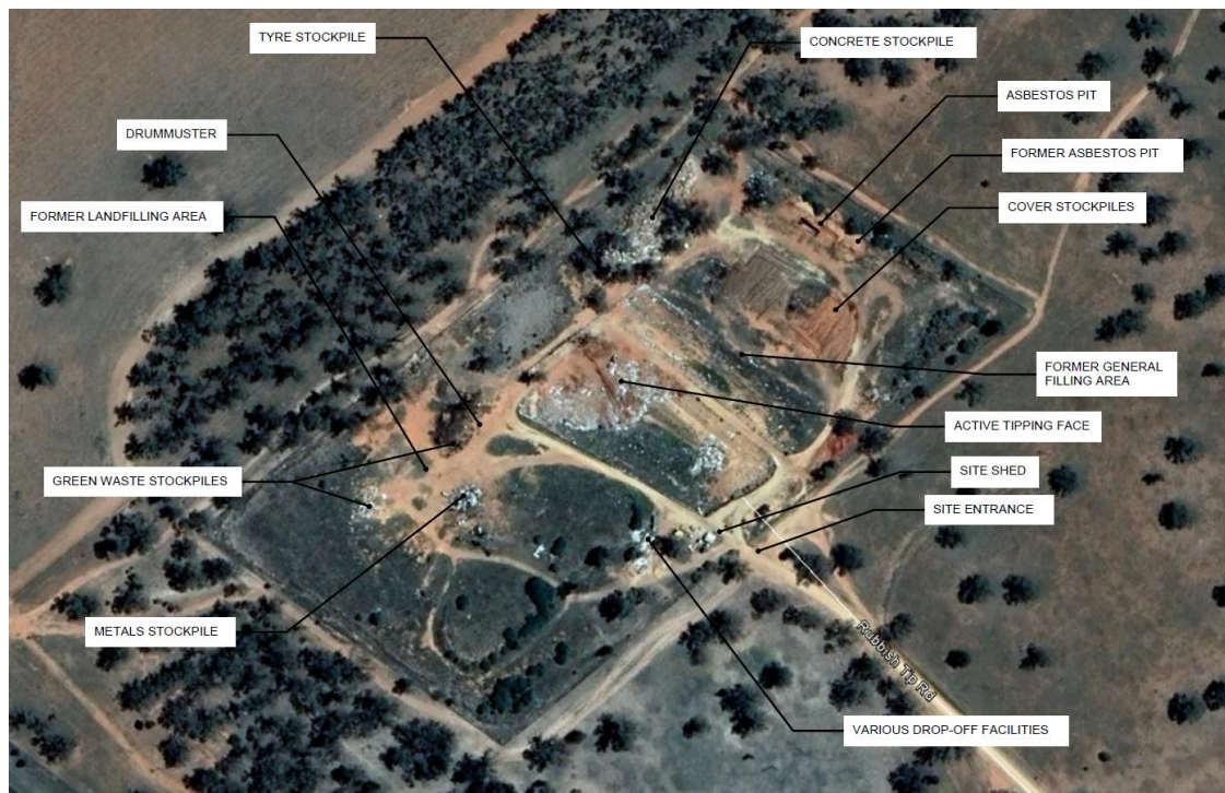
Figure 4.2 Trangie WMF existing site layout
