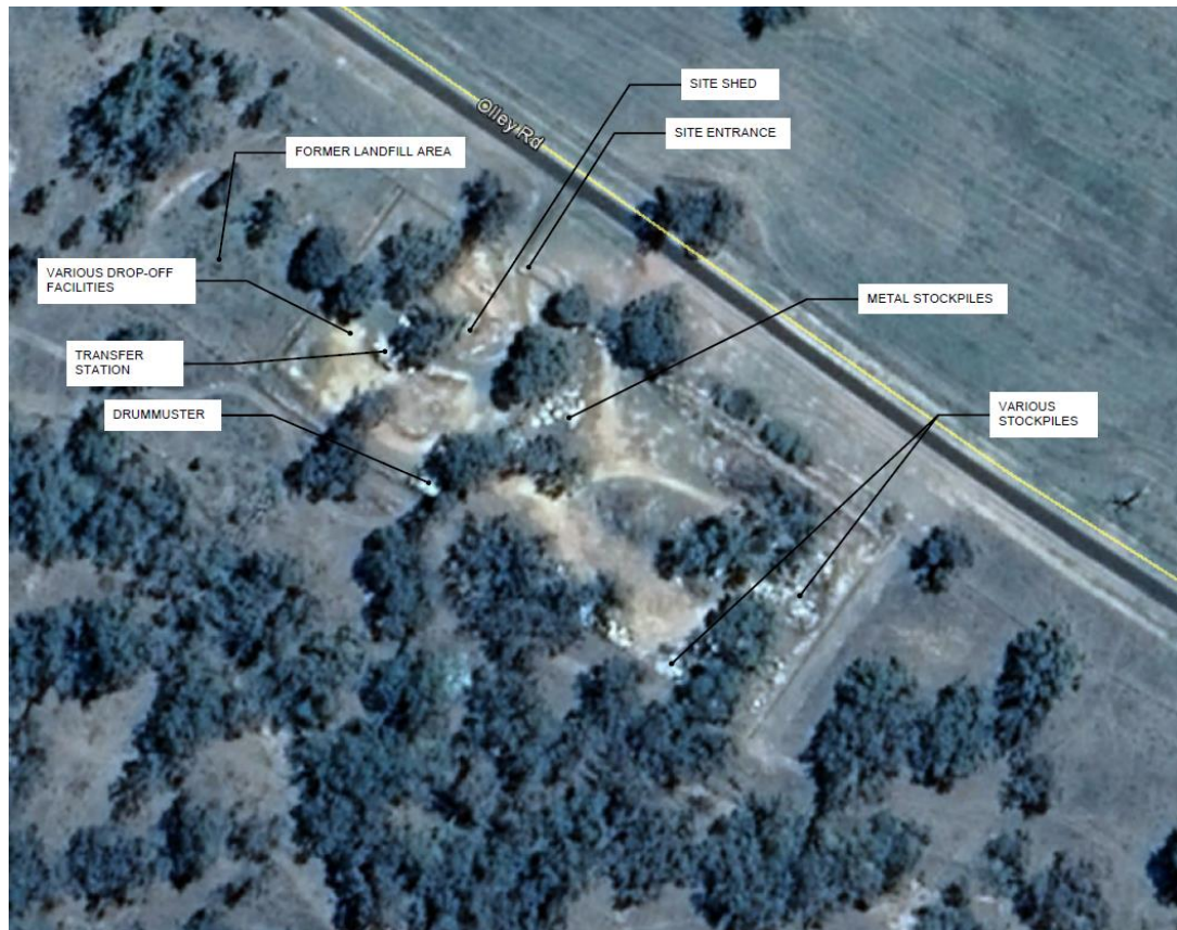
Figure 4.3 Tomingley Transfer Station existing site layout
